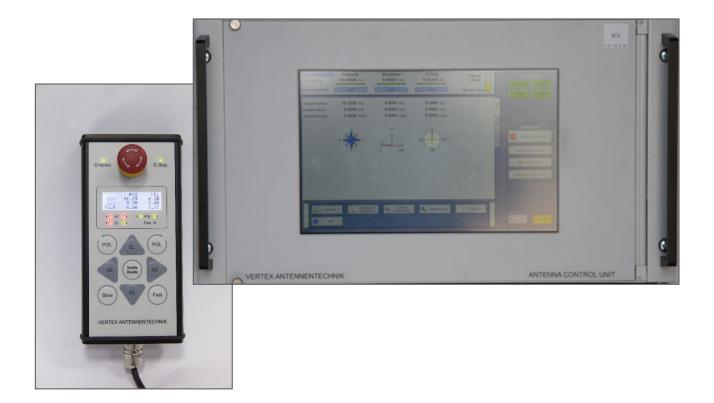
The Antenna Control Unit (ACU) 8100 Series, developed by Vertex Antennentechnik, is a state-of-the-art controller for antennas and pedestals. It has been particularly designed for antennas tracking low orbit satellites and for scientific and similar applications which require high precision and/or high velocity performance.
