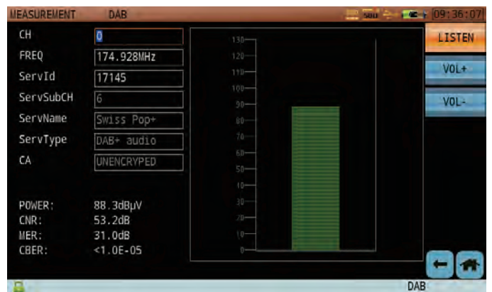
Figure 11: DAB Signal Measurement
