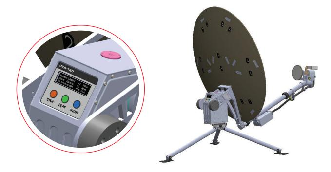
PROFEN's PTA-120M is a motorized transportable (Fly-away) satellite antenna designed for quick deployment and operation in VSAT applications. It is equipped with Profen's PAC750 series antenna control unit (ACU) with auto-acquisition, auto-peaking and satellite identification features to point the antenna to the predefined satellite.
