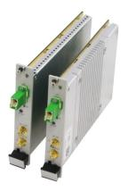
The Optiva OTS-1 Ref-100 Reference Oscillator Link is optimized for the transport of 100 MHz high-level reference signal input. It features low phase noise and high-dynamic-range, with optically-isolated DFB lasers that run cool and have low power consumption requirements.
