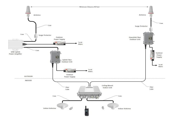
The Iridium re-radiating architecture consists of outdoor antennas connecting over fiber to an indoor unit which supports the connection of indoor Iridium re-radiating antennas. Phones connect wirelessly to the re-radiating antennas.
