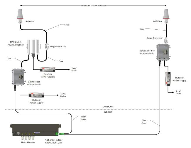
The Iridium direct connection architecture consists of outdoor antennas connecting over fiber to an Optical Zonu indoor unit that supports the direct connection of phones and/or data modems over copper media.
