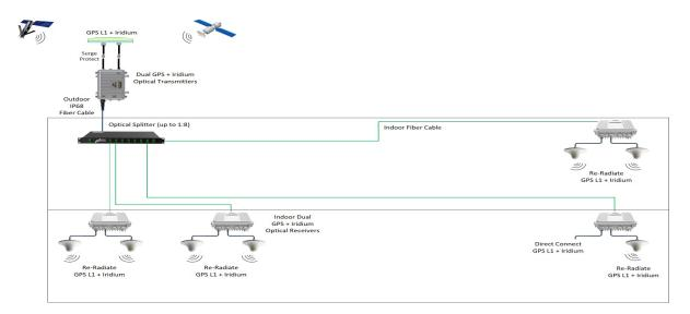
The Iridium paging + GPS architecture consists of a single receive only outdoor antenna that transports both Iridium paging plus L1 GPS to the appropriate indoor units.
