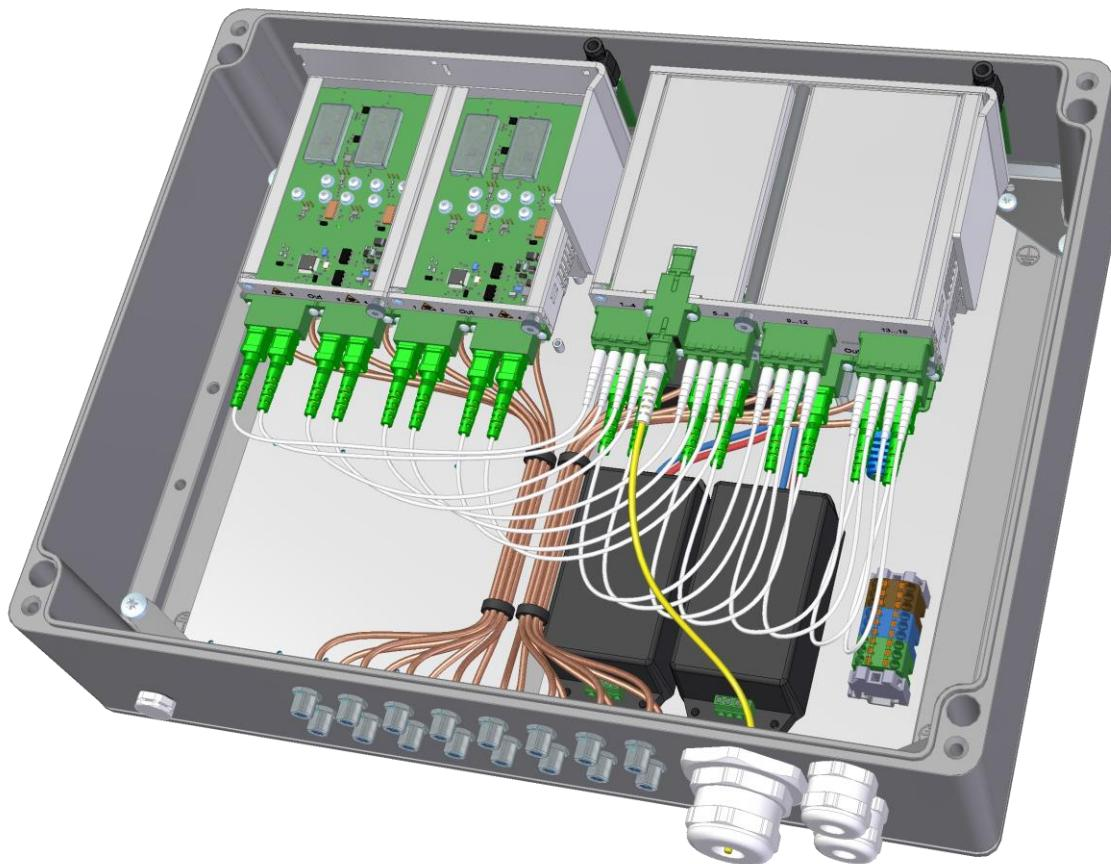
The DEV 7187 outdoor chassis can be equipped with up to four optical modules, i.e. up to 16 optical channels. The RF ports (with and without redundancy functionality) are installed below the optical modules. In addition, a slot located above the optical modules can be equipped with a CWDM de-/multiplexer. Optionally, the DEV 7187 can be equipped with a CPU for Monitoring and Control via Web Interface and via SNMP (Option 59).
