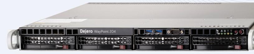
The WayPoint 204 receiver reconstructs broadcast-quality video transported over multiple IP connections from Dejero transmitters, decodes HEVC or AVC, and outputs to SMPTE ST 2110 workflows.
